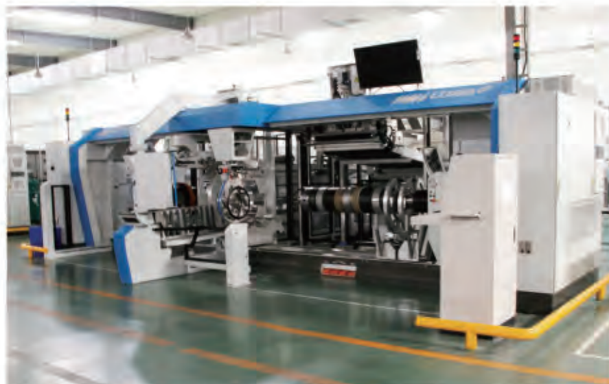
VMI EXXIUM building machine from Holland
